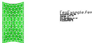
This gives us a comparison between the displaced shape and the original shape.
